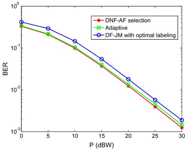
**Fig. 2** BER performance for DNF–AF selection scheme, adaptive two-way relaying, and DF-JM in Scenario 1
