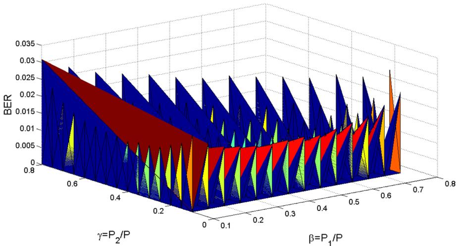
**Fig. 6** BER performance of the proposed DNF–AF selection scheme with general power allocations among the two sources and relay in Scenario 1, the total power is  $P = 20$  dBW
