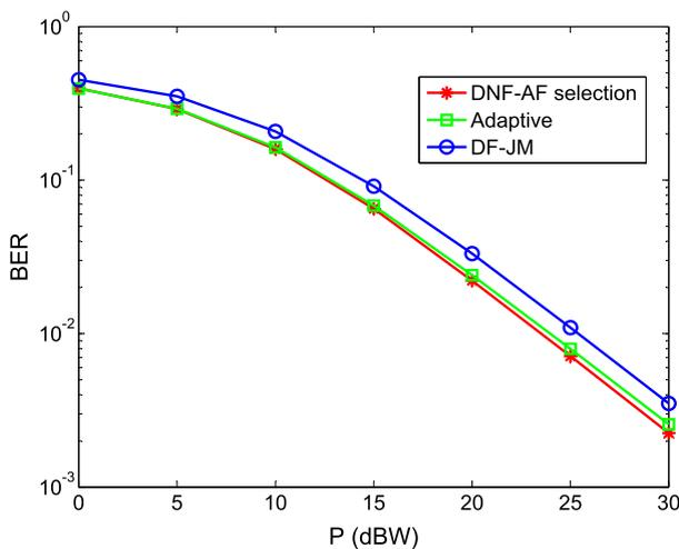
**Fig. 3** BER performance for DNF–AF selection scheme, adaptive two-way relaying, and DF-JM in Scenario 2
