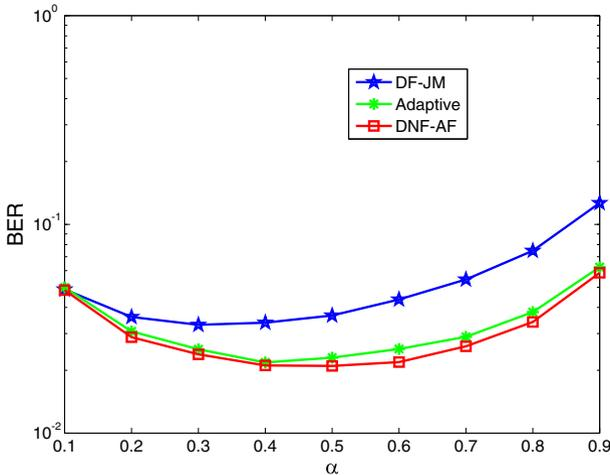
Fig. 5 BER performance with different power allocations in Scenario 2, the total power is  $P = 20$  dBW
