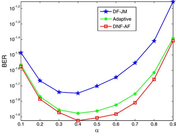
Fig. 4 BER performance with different power allocations in Scenario 1, the total power is  $P = 20$  dBW
